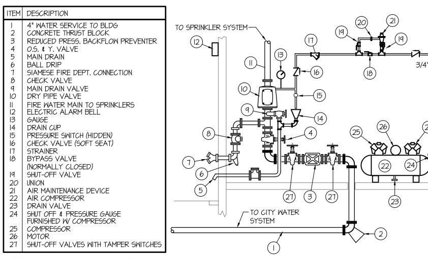
ALL PIPING THIS DETAIL TO BE INSTALLED BY FIRE SPRINKLER CONTRACTOR UNLESS NOTED.
